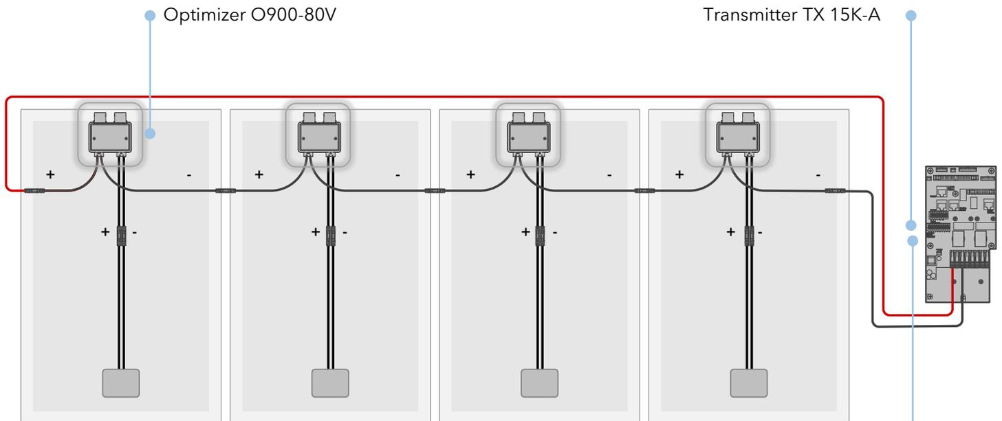
Figure (a) Basic configuration of O900-80V with TX 15K-A transmitters
