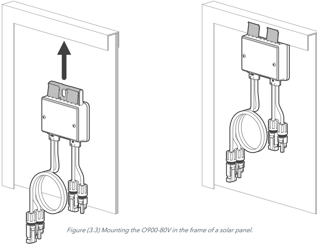
Figure (3.3) Mounting the O900-80V in the frame of a solar panel.
