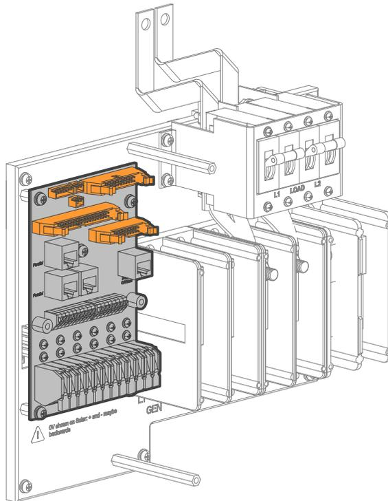
Carefully remove the four (12) M3 screws located at the top of the MPPTs terminals, then remove the remaining screws on the communications board.
