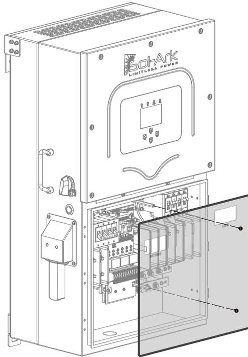
After installation of the TX 15K-A transmitter a rapid shutdown device must be installed. The Sol-Ark 15K-2P-N has the terminals to connect an emergency stop button, which must be easily accessible. Recommendation, place the emergency stop tag within 1m(3ft) of the emergency device. Always follow your local codes.
