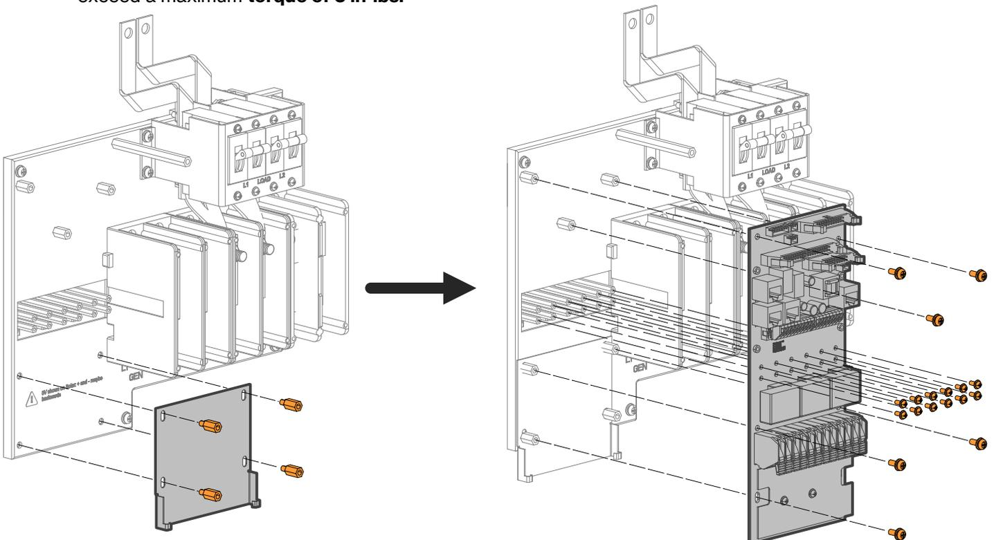
To install the plastic cover into position, use the extra 50mm standoff included in the installation pack to secure the board at the bottom.
